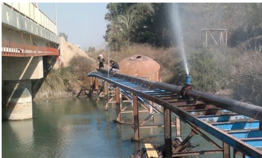
Figure (3): Suspended sediment sampling in Al- Diwaniyah River and its branches.
