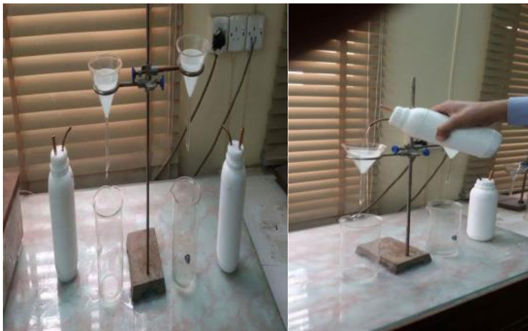
Figure (2): Home – made suspended sediment sampler locally manufactured.
