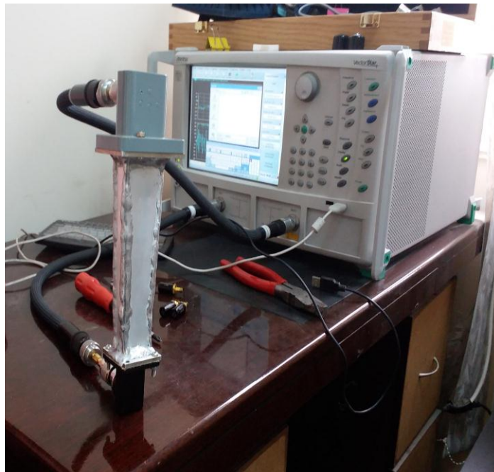
Figure 10: Waveguide taper test setup using two port network analyzer.
