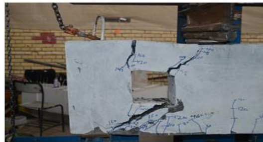
Figure (14) Crack Pattern for Beam CBO at Failure Load
