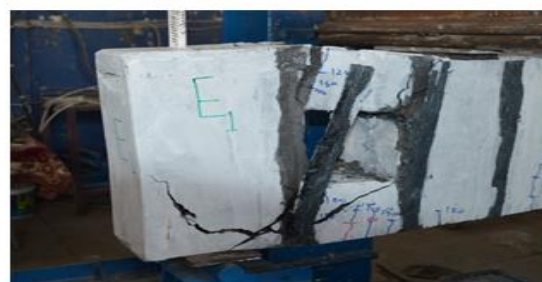
Figure (15) Crack Pattern for Beam SBE1 at Failure Load
