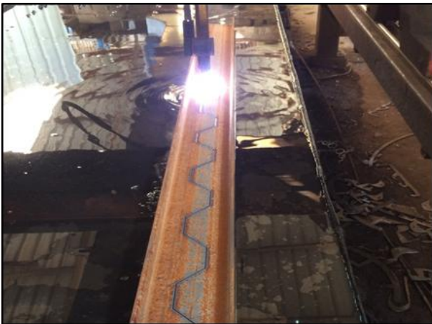
Figure 2: Thermally Cutting the Web of a Hot-rolled Parent Section for Tested Specimen
