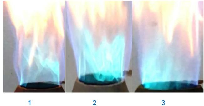
Figure 6. Photos of Burner with Conical Cup Confinement flame in premixed Combustion mode  $\dot{m}_f = 0.185 \text{ g/s}$ ,  $\dot{m}_a = 3.3 \text{ g/s}$ ,  $\phi = 0.85$
