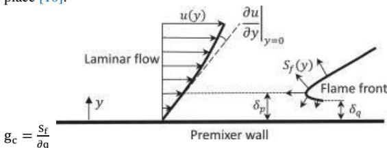
**Figure 1. Schematic Diagram of Boundary Layer Flashback**
