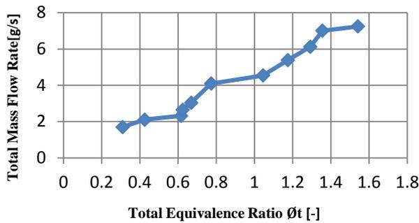
**Figure 8. Flashback Limits of Open Flame Burner in Partial Premixed Combustion Mode.**
