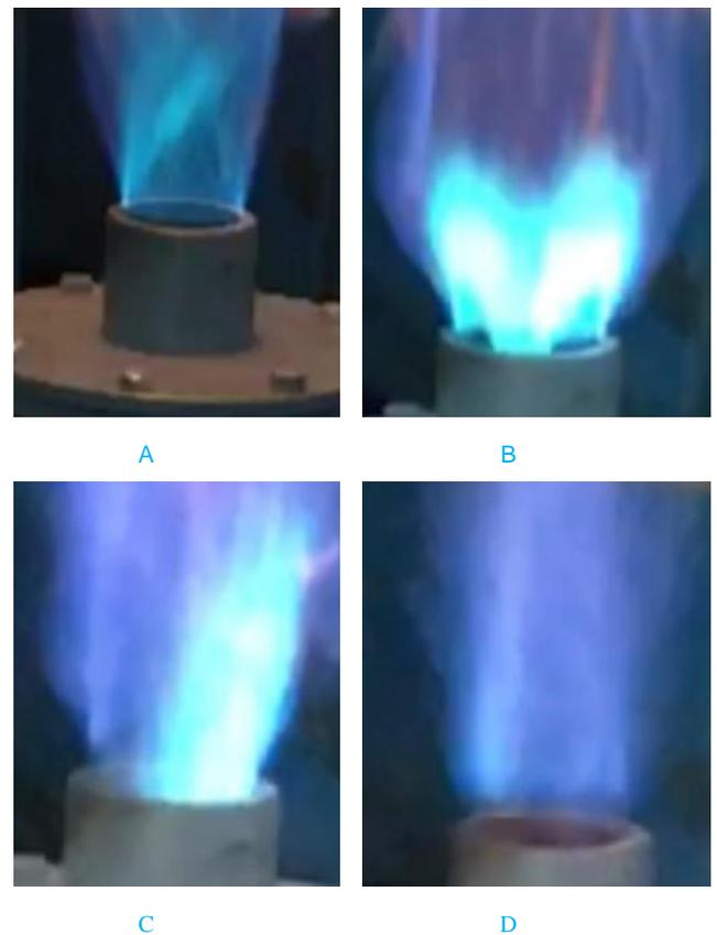
Figure 3. Photos of Open Flame Burner in Premixed Mode  $\dot{m}_f = 0.046 \text{ g/s}$ ,  $\dot{m}_a = 2.4 \text{ g/s}$ ,  $\phi = 0.29$
