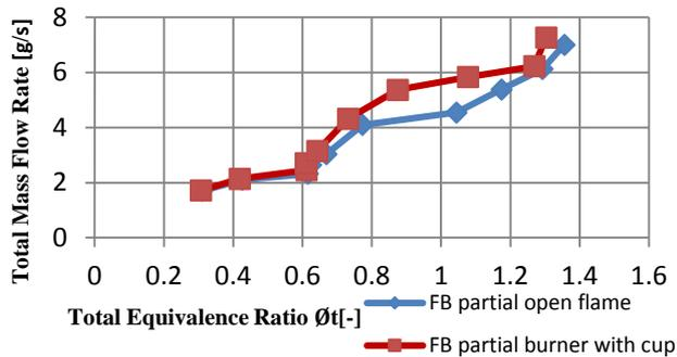
**Figure 9. Flashback Limits Comparison of Open Flame Burner and Burner with Conical Cup Confinement in Partial Premixed Combustion Mode.**
