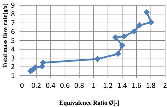
Figure 4. Flashback Limits of Open Flame Burner in Premixed Combustion Mode.
