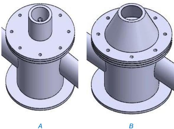
Figure 2. (A) Open flame burner. (B) Burner with conical cup confinement.
