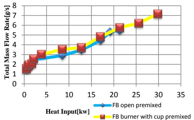
Figure 7. Flashback Limits Comparison of Open Flame Burner and Burner with Conical Cup Confinement in Premixed Combustion Mode as a Function of Heat Input and Total Mass Flow Rate.
