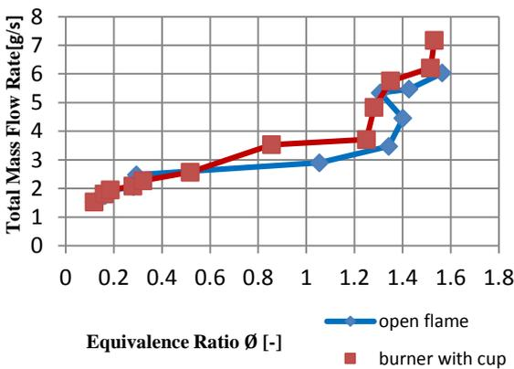
Figure 5. Flashback Limits Comparison of Open Burner and Burner with Cup in Premixed Combustion Mode.
