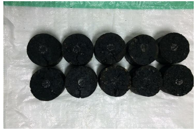
Figure 6. Specimens after Double Punching Test.
