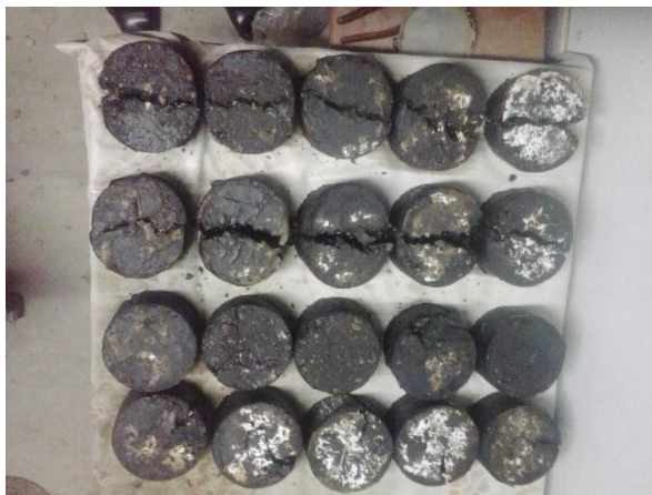
Figure 5. Specimens after ITS Test.
