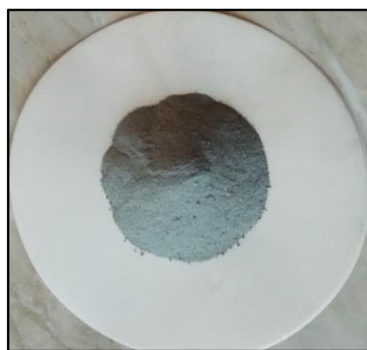
Figure 2- The prepared CoMo/Al_2O_3 catalyst powder after calcination.
