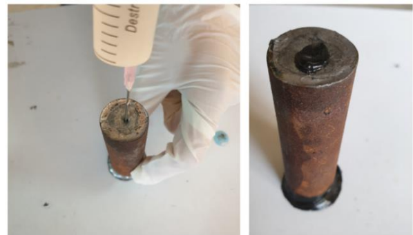
Figure 3. Injecting melting paraffin wax in capsule.
