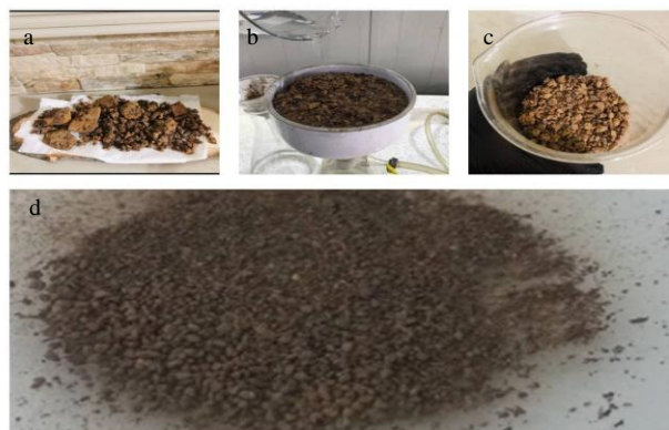
Figure 3. Photographic picture of the steps of preparation of polymer. a. The polymer was broken into large spatula; b. The polymer was rinsed in DI water many times; c. A mechanical mill was used to grind the polymer into particles ranging in size from 0.5 to 3 mm; d. The produced polymer was dried in the sieve by putting the material in drying oven at 42°C.
