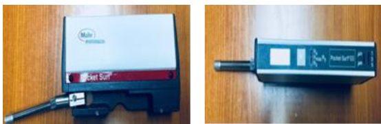
Figure 4. Surface roughness measuring device
