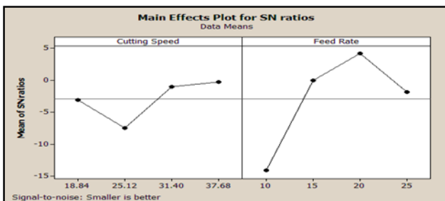
Figure 8. Main effects plot for S/N ratios on surface roughness for UP cut milling on fluid machines.
