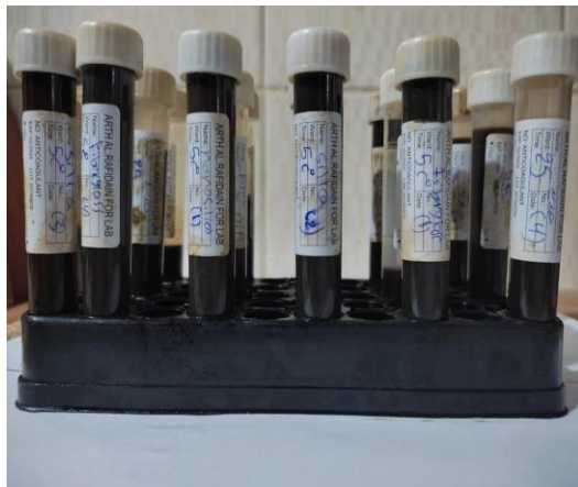
Figure 6. Separation of asphaltenes from the crude oil.
