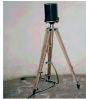
Fig. 4. Electronic equipment ( top ) and the three-axis fluxgate sensor ( bottom ) for the land stations.
