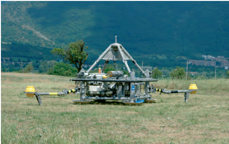
Fig. 5. GEOSTAR submarine module (frame) at L'Aquila during calibration and comparison with magnetic data from observatory. Magnetometers are mounted at the extremity of the oppositely extended booms.
