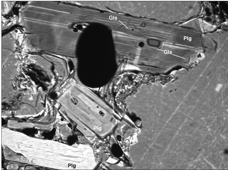
Fig. 1. Microscopic image of a chemically zoned plagioclase phenocrysts (Plg) in a highly vesicular pumice sample from the Minoan Tuff (Santorini, Greece). Inclusions in the plagioclase host represent quenched melt (Gls) trapped at various stages during crystal growth and thus provides information on the compositional development of the erupted magma (Large black spot: Vesicle filled with resin above Plg-crystal). Bottom side of image 1.2 mm, crossed polarizers).
