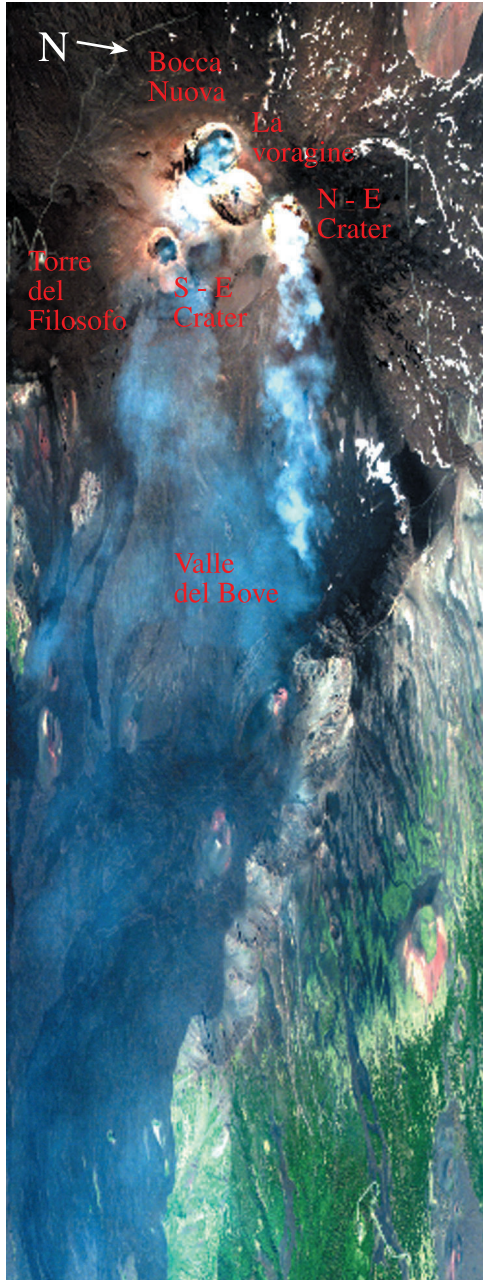
Fig. 2. MIVIS image Etna June 16th 1997 calibrated in Radiance RGB composition. Flight altitude 6000 m. Pixel resolution ranges to 4 \times 4 \text{ m}^2 at summit craters to 11 \times 11 \text{ m}^2 at the sea level.
