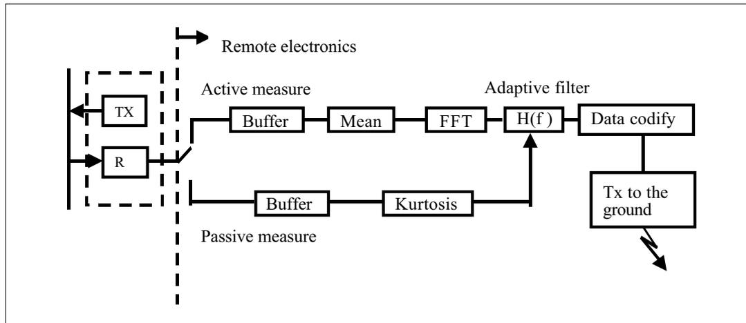
Fig. 3. Data processing block diagram.
