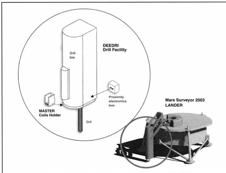
Fig. 1. Allocation of the TDEM instrument on board of DEEDRI.
