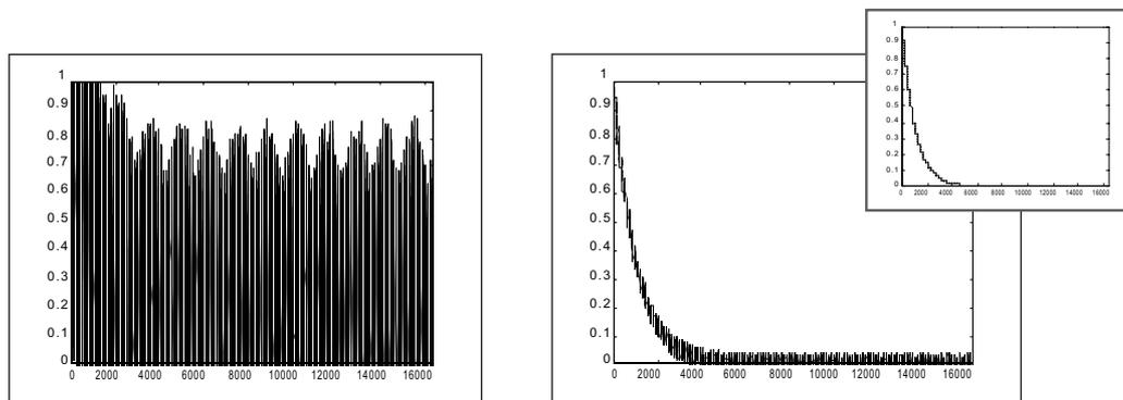
**Fig. 5.** Simulation results. On the left side: the received signal  $r(t)$ . For the test the noise was modelled as the sum of two sinusoids with a maximum amplitude equal to 0.6, an AWGN with a maximum amplitude equal to 0.2 and a spike with a maximum amplitude equal to 0.3 and a duration of  $500 \mu\text{s}$ . On the right side: the processed signal obtained after filtering and compressing procedures; in the small window: the original signal  $s(t)$ .
