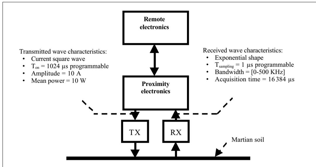
Fig. 2. Scheme of the TDEM system designed for DEEDRI.
