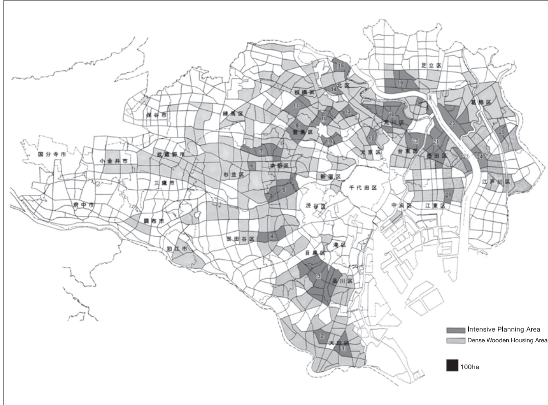
Fig. 4. Dense wooden housing areas and intensive district for Safe Living Environment Zone Project in Tokyo (Tokyo Metropolitan Government, 1996).
