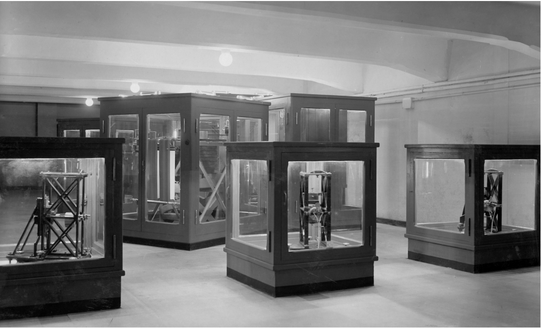
Fig. 2. Galitzin seismographs installed at Roma seismic station (1939).
