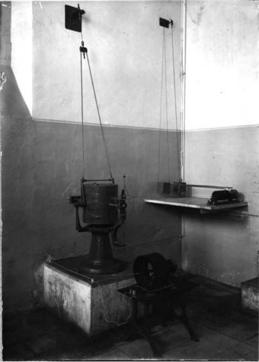
Fig. 2. The Grablovitz pendulums (right) installed at the seismic pavilion of the Ebre Observatory (circa 1915). The larger seismograph in the center of the photograph is the Mainka-Ebre instrument, constructed at the Ebre Observatory (copy of the original photograph preserved at the Ebre Observatory Archive).
