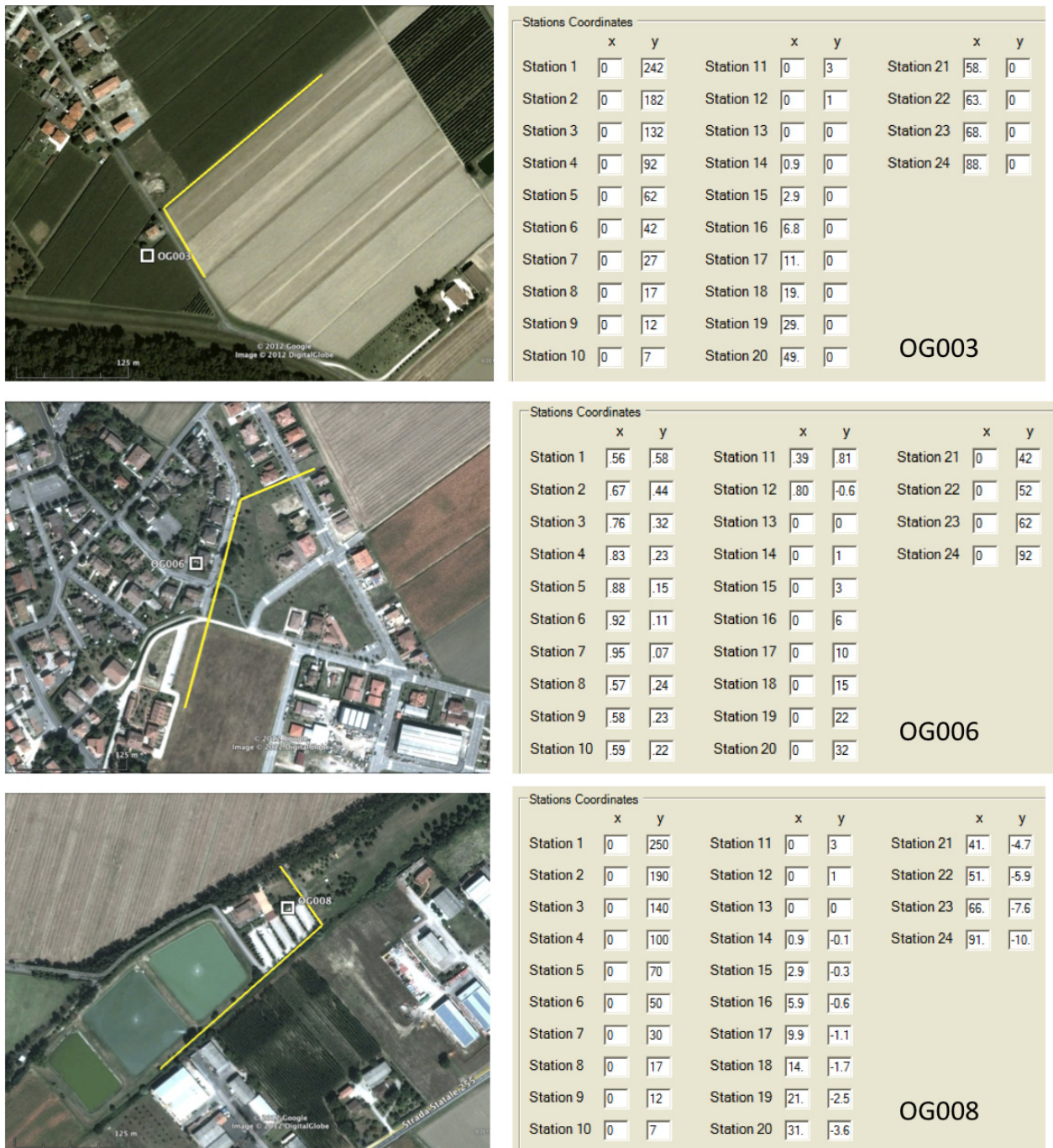
Figure 6. Array geometry (yellow lines) of the ESAC surveys performed at the OG003, OG006 and OG008 sites. For each site, a map and a list of the geophone coordinates are shown. The location of the temporary station is indicated by a white square in each map. The array geometry consists of two nearly orthogonal branches. The array length specified in the text is the total length of the two branches.
