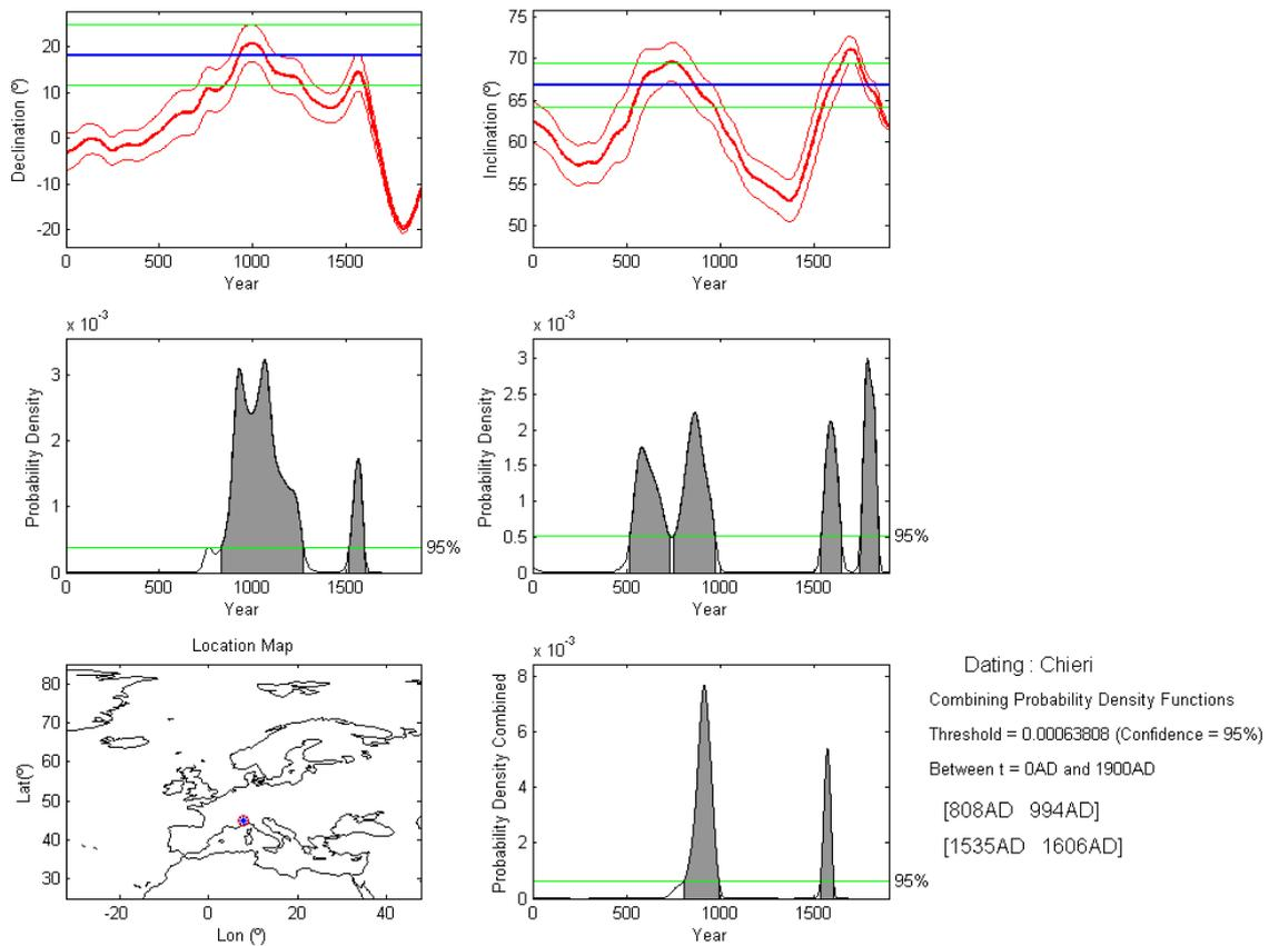
**Figure 6.** Archaeomagnetic dating results. Up: declination (left) and inclination (right) reference secular variation curves calculated from the SCHADIF3K model (red curve with error band) and the kiln's measured direction (blue line with green error band); middle: calculated probability density functions for declination (left) and inclination (right); down: combined probability density function for declination and inclination.
