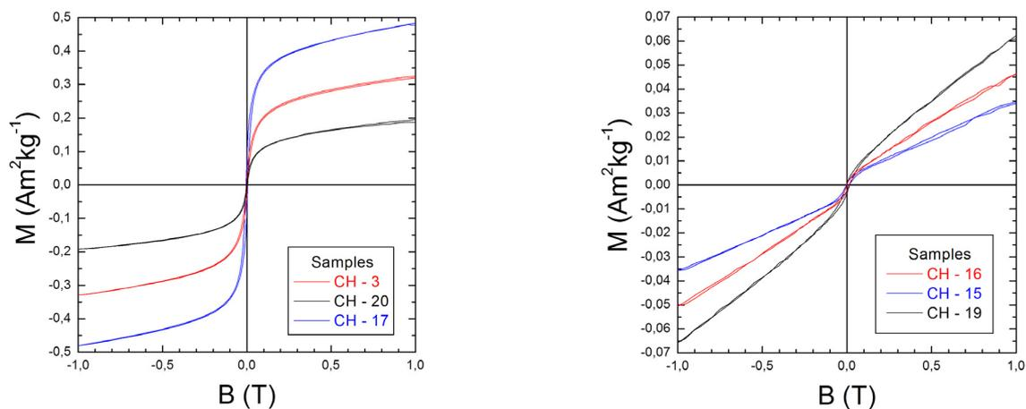
**Figure 2.** Hysteresis cycles for representative samples. Two main groups are individuated according to their magnetic behavior: presence of SD and PSD plus minor superparamagnetic grains (left side) and dominant paramagnetic grains plus faint SD and PSD contributions (right side).
