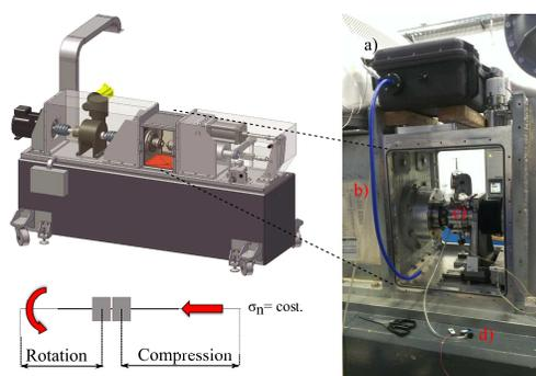
**Figure 2:** The experimental apparatus (SHIVA, on the left modified from [Di Toro et al.(2010)]) essentially made of a rotary axes, a stationary axis and a sample chamber. The experimental assembly consists of the radon detector. (labelled with a), the connection (b) allowing for close loop circulation of fluids from the vessel (c) to the radon detector.; the air pump for air flux (d).
