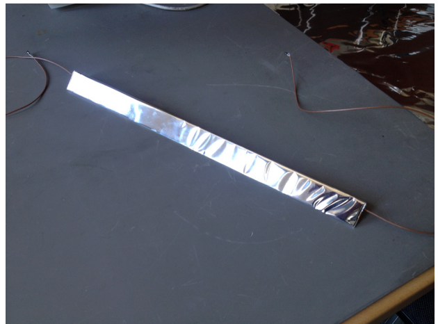
Figure 10. One scintillator bar enveloped in the aluminized mylar film.
