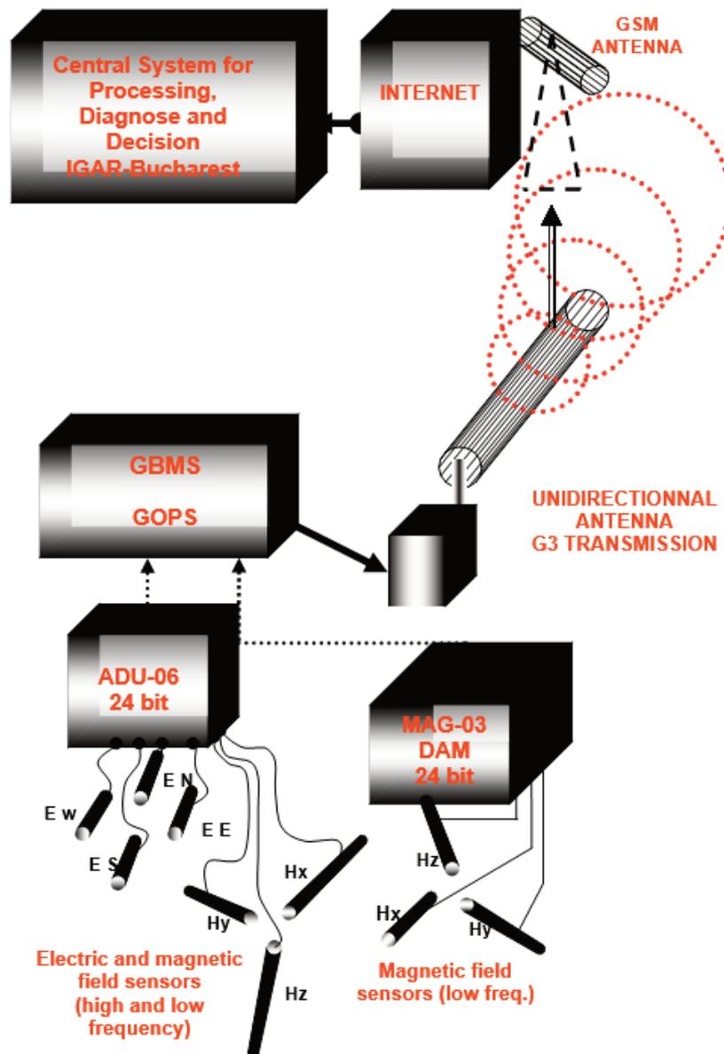
Figure 1. EM monitoring system, data transfer and central computer for real-time data processing and analysis.
