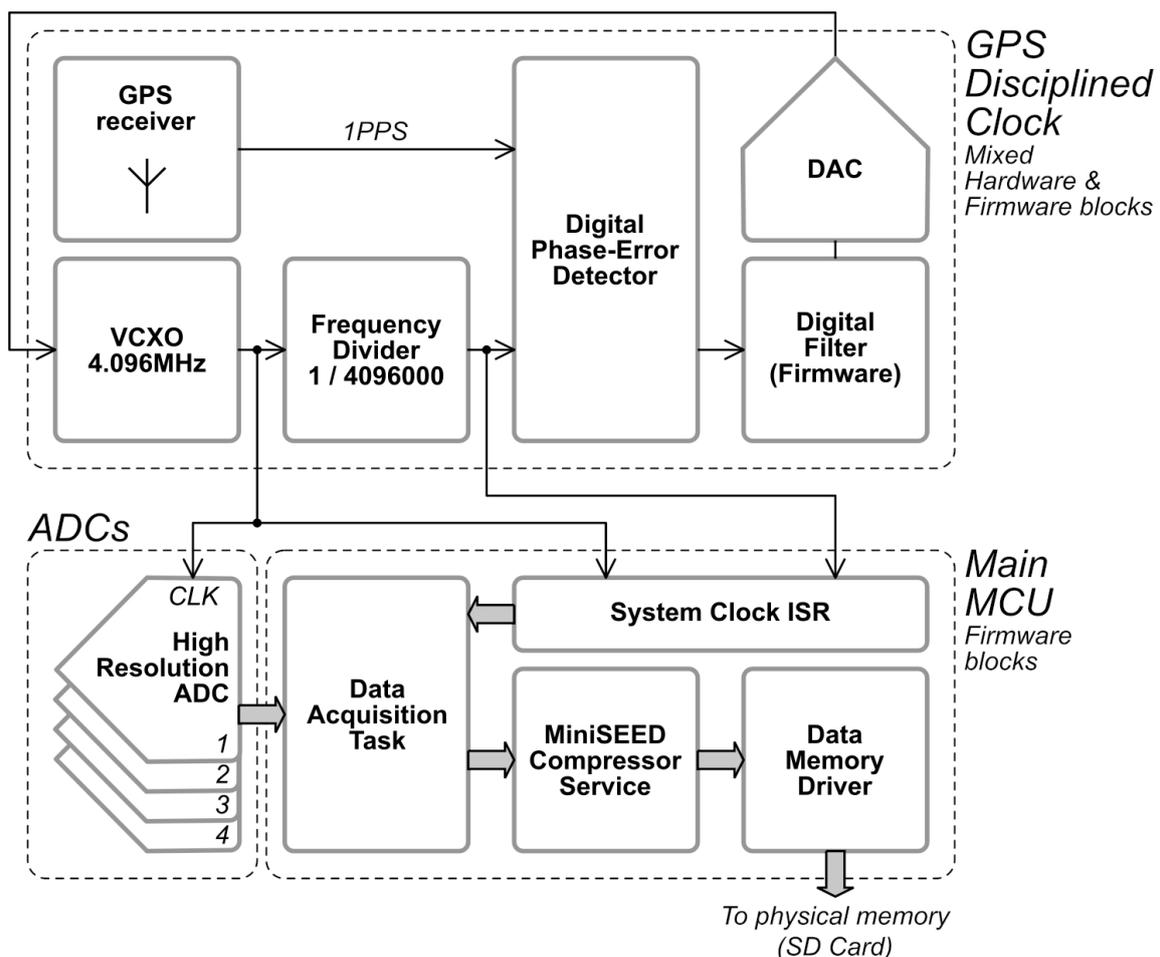
Figure 6. Clock distribution network of the SeismoLog Recorder.
