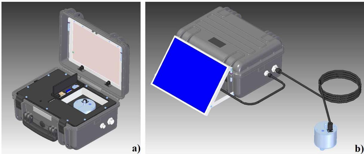
**Figure 1.** 3D assembly model of PGS1; a) transport configuration (with open suitcase and without pocket), b) acquisition configuration.
