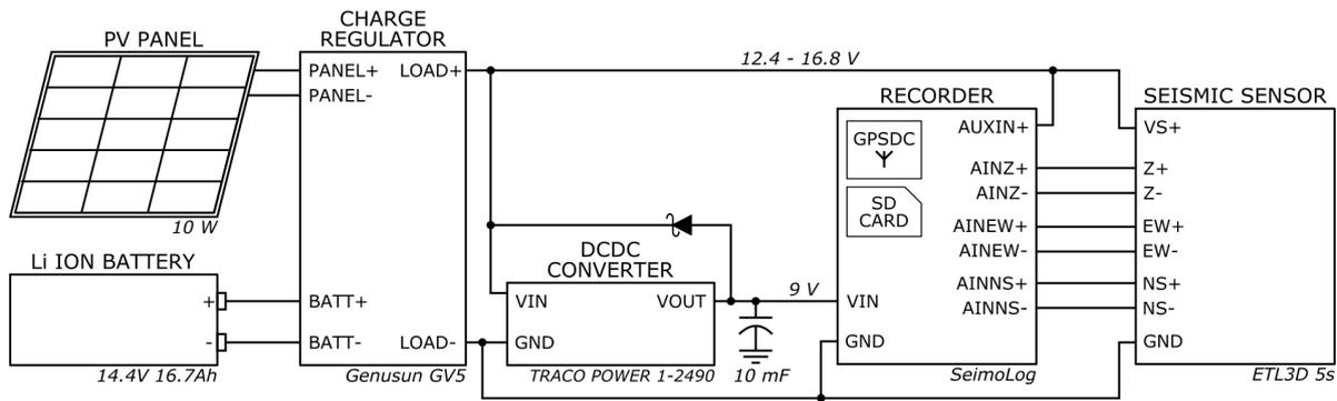
Figure 7. PGS1 schematic diagram.
