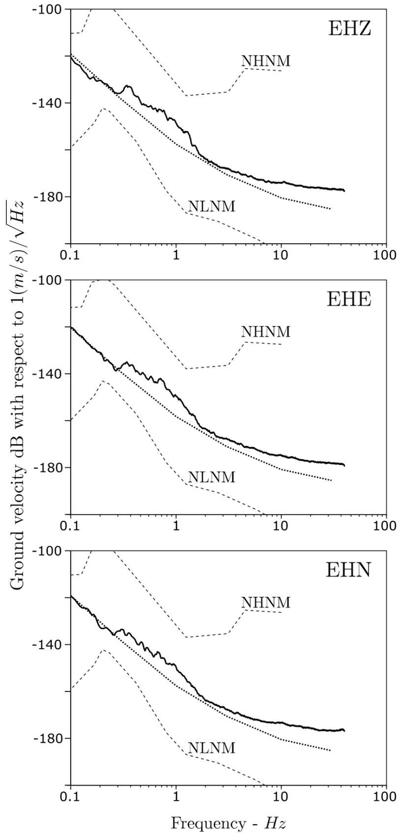
**Figure 12.** Component spectra of a data segment, recorded by PGS1 n° 06. The dotted curve is the sensor's self-noise, as resulted from a simulation; the dashed curves are the Peterson models, high and low; the continuous curve is the measured spectrum.
