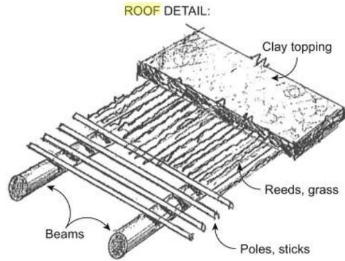
Figure 4: Technique of roof construction
