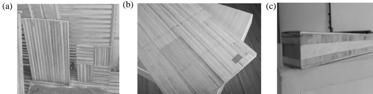
Figure 5. (a) Samples cut out from DPLM board , (b) DPLM board after treated (c) DPLM double board as a sandwich panel.
