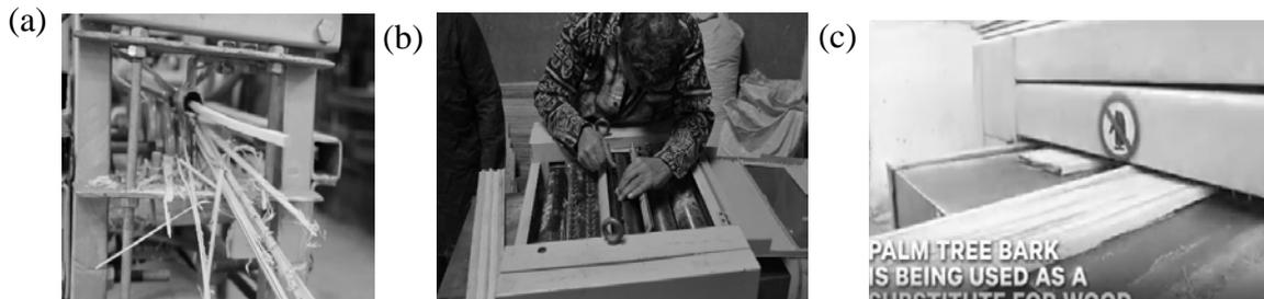
Figure 6. Photographs of (a) Cutting process, (b) Trimming process (c) Collect and Compress process.
