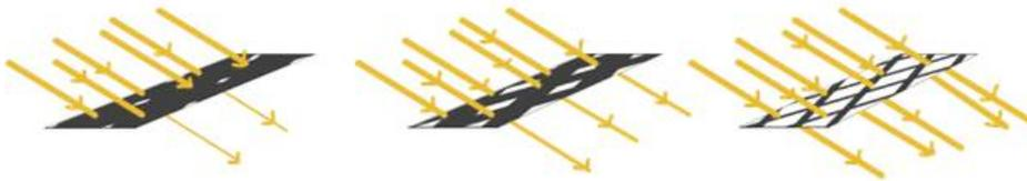
Fig.2 Control over the amount of light depending on pattern size
