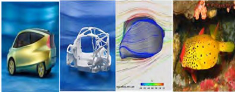
Figure 4. Daimler Chrysler car design inspired by the shape of a fish and the way trees grow.
