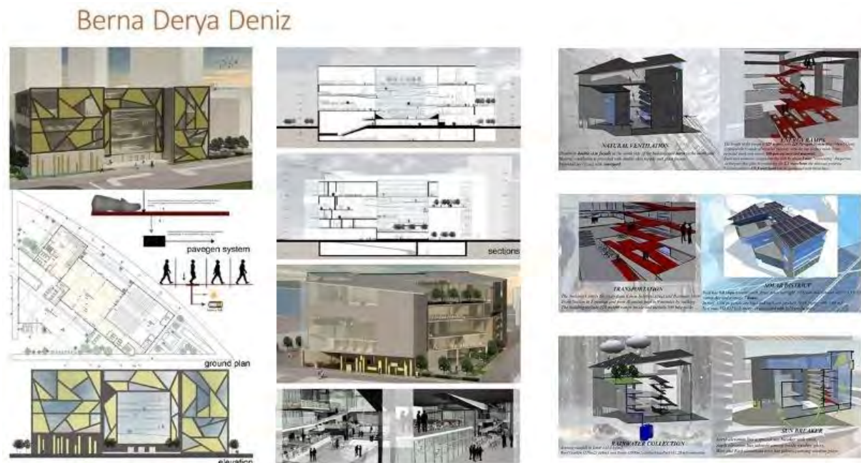
Figure 2. The designed Architecture school incorporate the use of; long ramps floors to convert kinetic energy to electricity, natural light, shading elements, natural ventilation, solar panels, green roof, rain water collection.
