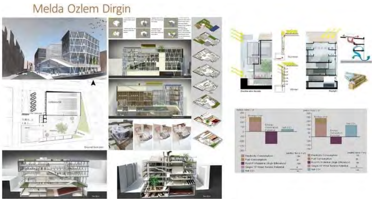
Figure 4. The designed Architecture department project incorporate the use of; natural light, natural ventilation with wind catchers, sustainable materials (constructed out of wood and steel), double skin façade, shading elements, green roofs, collecting rain water, reuse of grey water, and solar panels. The proposed design had %32 reduction in annual energy consumption
