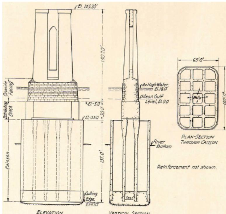
Figure 4. The various components of caissons
