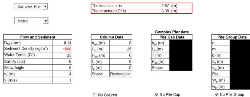
Figure 16. Scour depth calculation using FDOT program.
