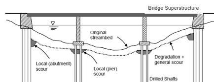
Figure 1. The scour around bridge supports (FHWA, 2010)
