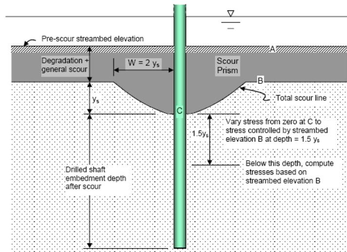
Figure 2. The effect of scour on bridge foundations (AASHTO LRFD Bridge Design Specifications, 2007).
