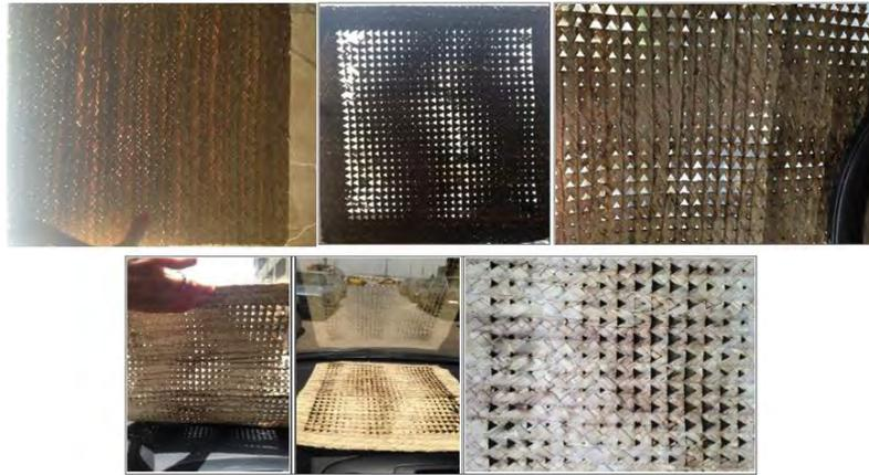
Figure 16. Palm leaves mat before and after laser cut and how it helped to change the users perception to the material.
