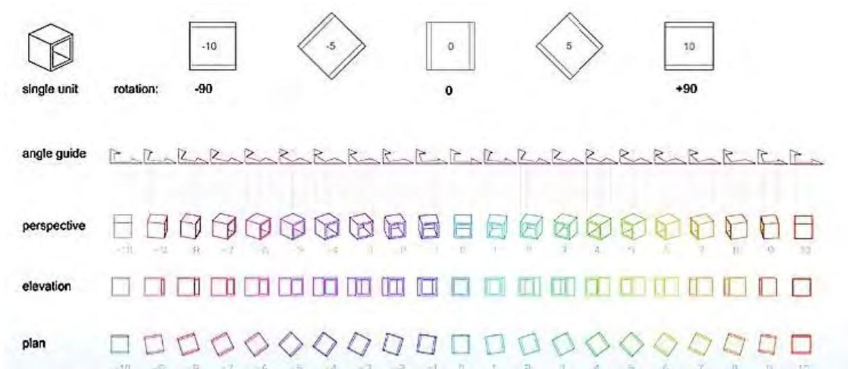
Figure 6. SilkWall. The angles of rotation of the cement blocks were constrained to 21 values. Wooden formats were given by the architect to educate the manufacturer show to distribute the pieces to the right position.
