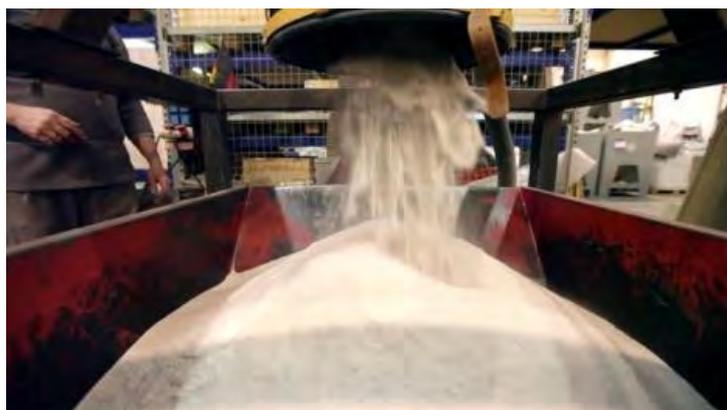
Figure 13. The excessive sands while printing process
