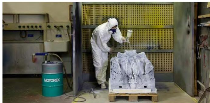
Figure 12. The finishing coat.
