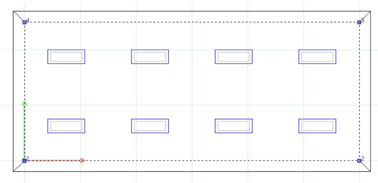
Figure 4. Luminaire Distribution Using DIALux
