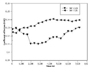
Figure 1c. Coefficient of friction (COF) at 125 °C
