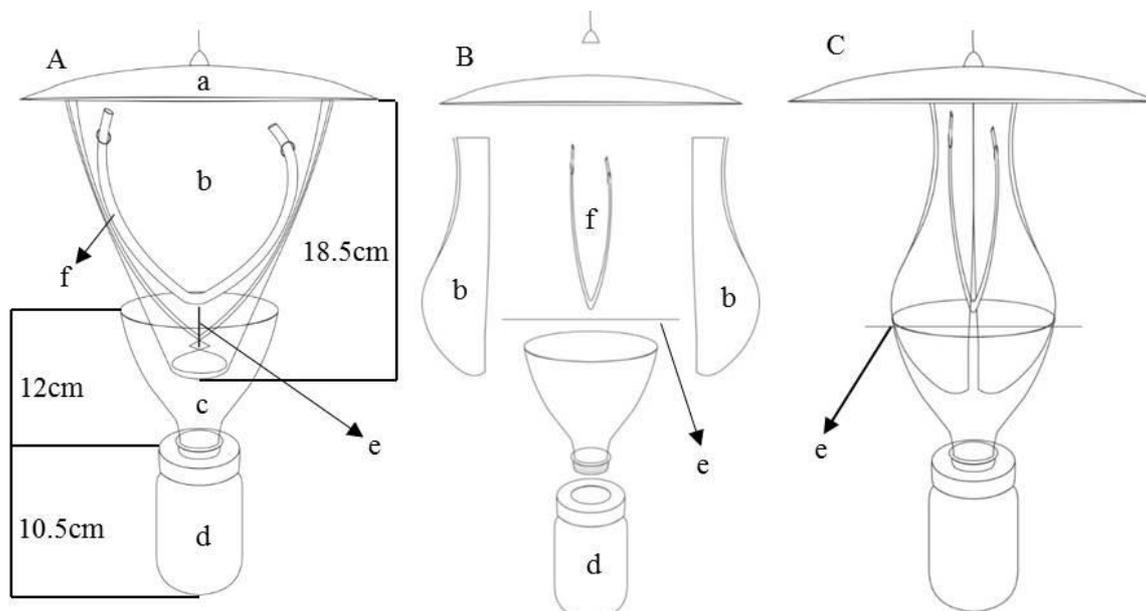
**Figure 1.** A – Front view: (a) Protection plate; (b) “Semi-funnel” interceptor panel; (c) Collector funnel; (d) Storage bottle; (f) Baitholder hose; (e) Fixing wire; B – Side view of parts: (b) Interceptor panel; (e) Fixing wire; (f) Baitholder hose; (d) Storage bottle; C – Side view of the installed trap: (e) Fixing shaft (rigid wire). Source: Carvalho and Trevisan (2015).
