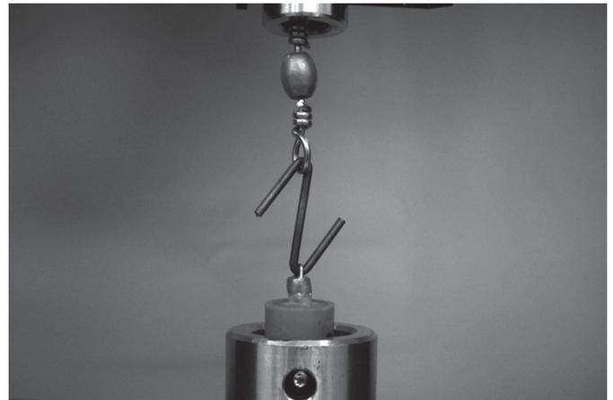
Fig. 5 - Specimen positioned in the testing machine.
