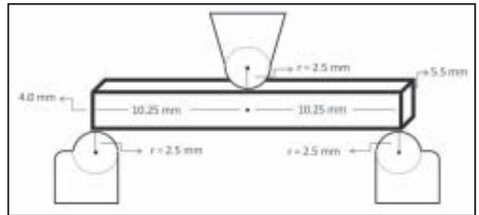
Figure 2 – Flexural strength test schematic's representation.
