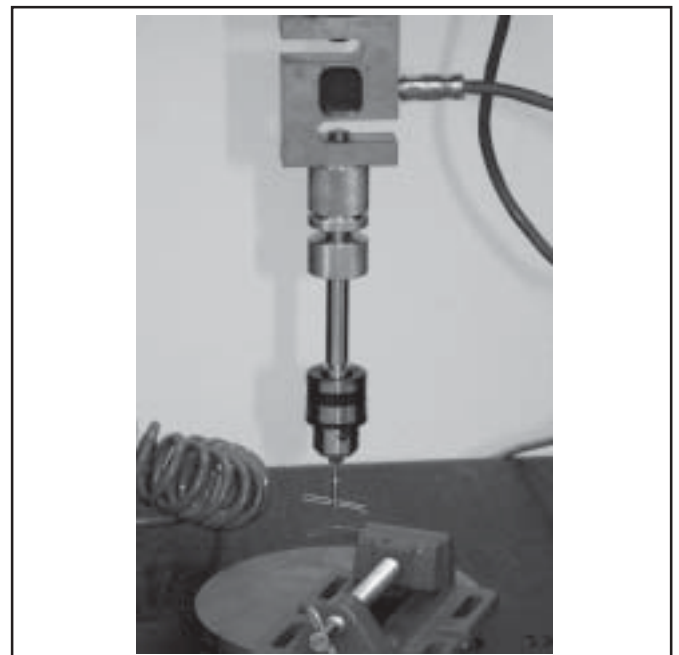
Figure 2. W-arch subjected to 12-mm compression in the EMIC DL 10000 testing machine.
