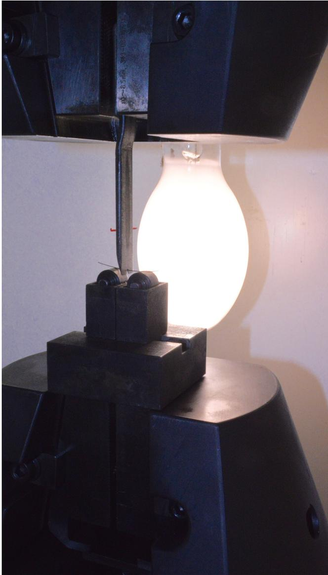
Fig. 1 - Specimen positioned for three-point bending test at 37 °C.
