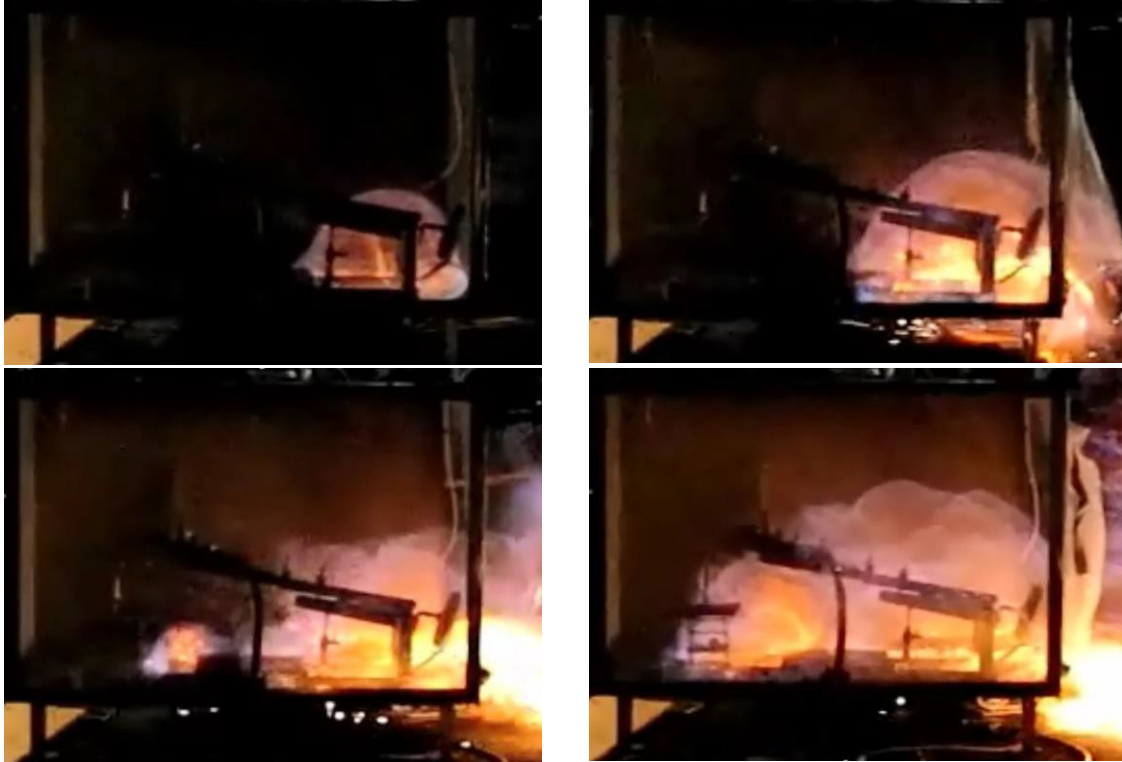
Figure 1: Example of a Raleigh-Taylor instability developing in a 1.5 \text{ m}^3 vented chamber (stoichiometric hexane- air). Top left: vent opens, flame surface drawn in direction of vent opening (towards the bottom right) and stabilises. Top right: pressure in chamber close to atmospheric. Flame starts to accelerate into chamber towards heavier unburned vapour-air mixture. Bottom left: Raleigh-Taylor instability causes large flame evolutions on flame surface causing further flame accelerations. Bottom right: development of flame evolutions continues.
