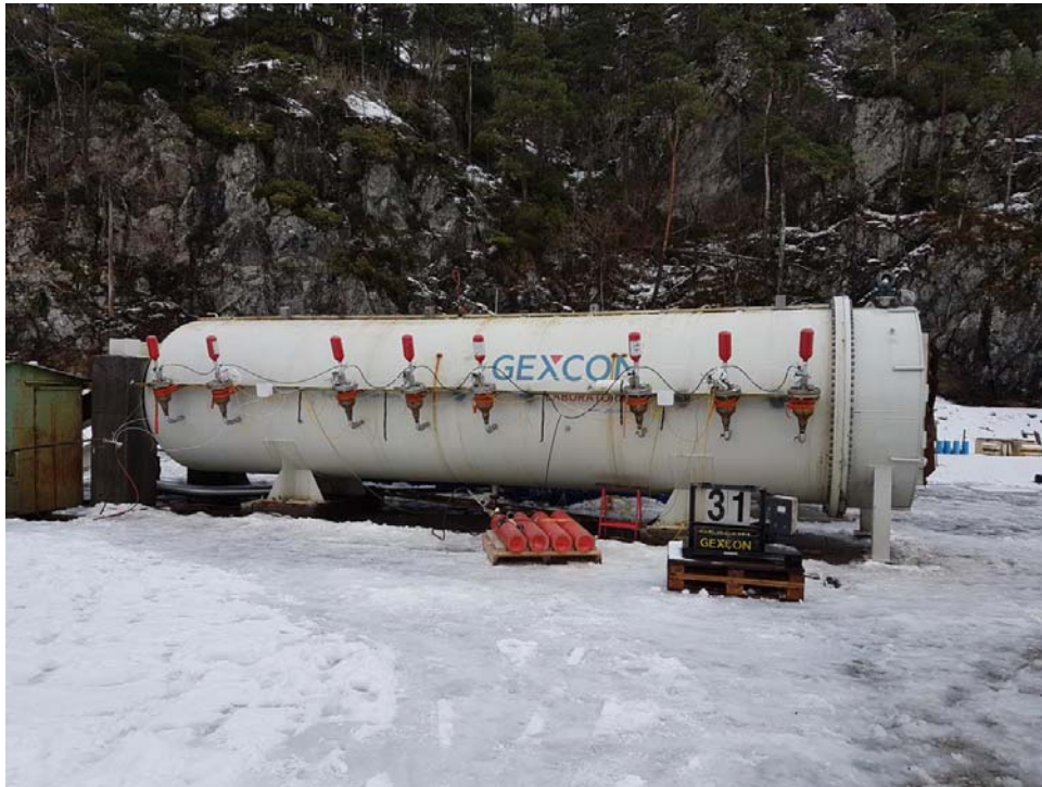
Figure 4: 55 m 3 elongated vessel provided with 8 dust injection bottles.
