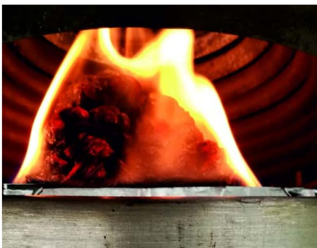
Figure 2: Swollen char layer formed on the surface of myo-inositol sample.
