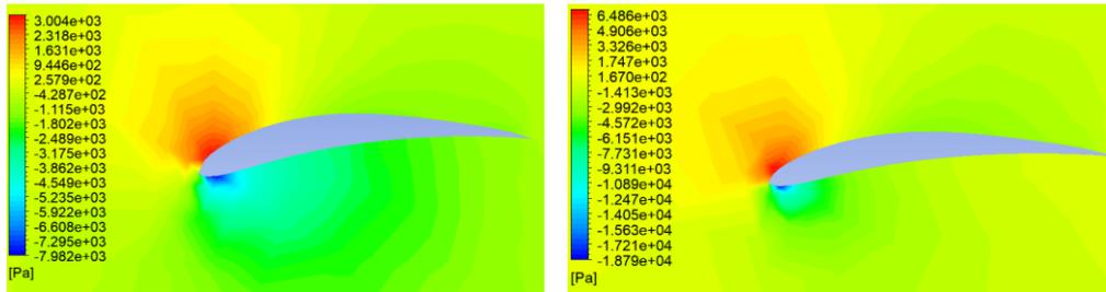
Figure 5: Pressure contours for stations 2(left) and 3(right)
