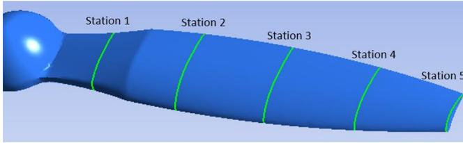
Figure 3: Selected stations along the propeller spanwise direction
