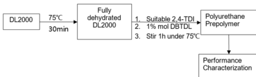
Figure 1: Flow chart for polyurethane prepolymer preparation
