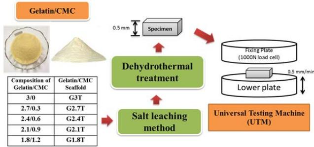
Figure 1: Schematic diagram of salt leaching gelatin/CMC scaffold preparation and experimental test.
