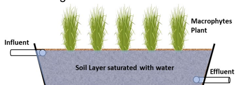
Figure 3: Schematic diagram of subsurface slow constructed wetland
