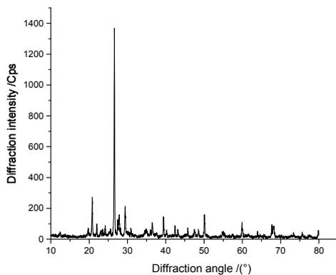
Figure 6: X-ray spectra of natural loess
