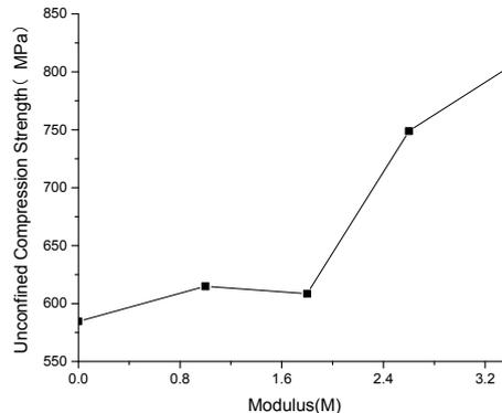
Figure 3: The effect curve of modulus
