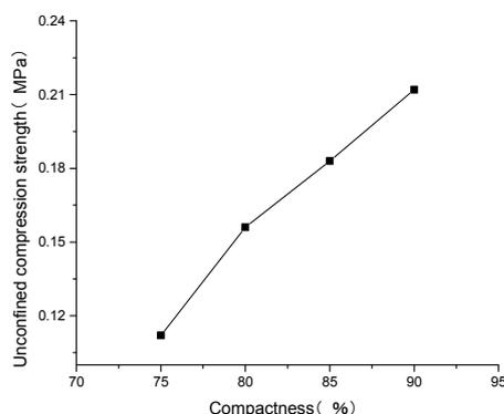
Figure 1: Relationships between unconfined compression strength and compactness
