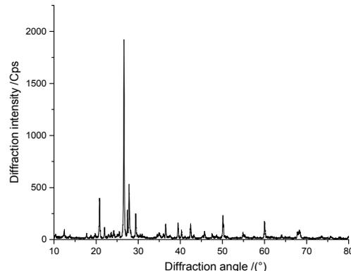
Figure 7: X-ray spectra of improved loess
