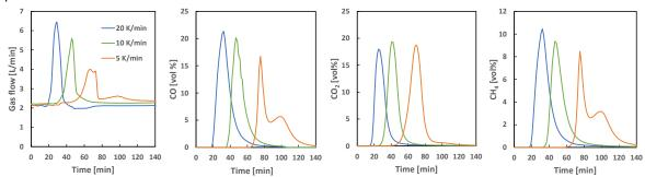
Figure 4: The gas flows (total, CO, CO<sub>2</sub> and CH<sub>4</sub>) during experiments 2 (20 K/min), 3 (10 K/min) and 4 (5 K/min)
