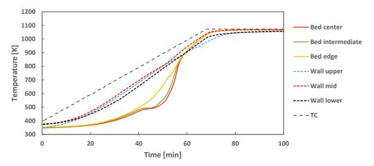
Figure 2: The temperature profile at the edge, an intermediate position, and the center position of the fuel bed, the control temperature of the three sections of the furnace (TC) and the temperatures of the outer reactor wall for experiment 1
