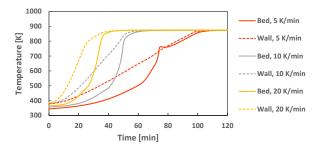
Figure 3: **Left**: The temperature profile during heat-up in the center of the pellets bed for experiments 1, 3 and 5, **Right**: The temperature profile during heat-up at the reactor wall and in the center of the fuel bed for experiments 2, 3 and 4 with heating rate 20, 10 and 5 K/min, respectively
