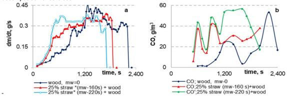
Figure 2: Effect of the increasing irradiation time for wheat straw pellets on the weight loss during the thermal decomposition of the 25 % straw (MW)\*+wood mixture (a) and on the yield of CO (b)
