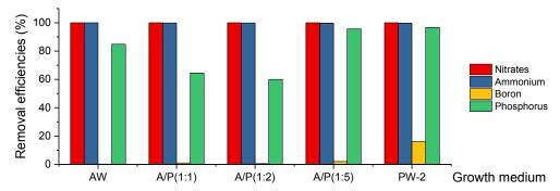
Figure 2. Effect of algae growth on the removal rate of relevant contaminants in the wastewaters
