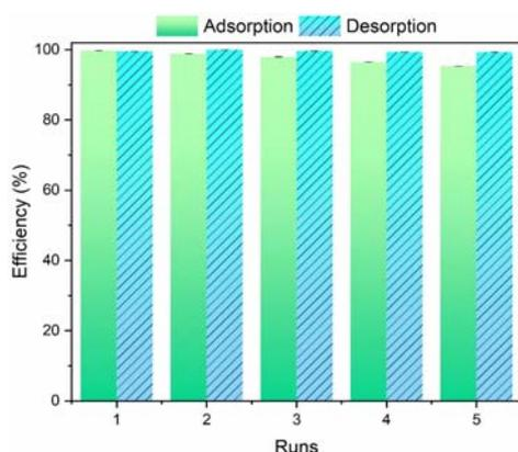
Figure 5: Adsorption-desorption of AMX onto and from graphene-OH at  $C_o = 80 \text{ mg L}^{-1}$ ,  $\text{S/L} = 10$ ,  $\text{pH} = 5$ , and  $T = 25 \text{ }^\circ\text{C}$ .
