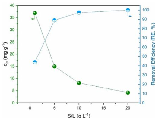
Figure 4: Effect of adsorbent dosage to the adsorption of AMX onto graphene-OH at varied solid to liquid (S/L) ratio,  $C_o = 40 \text{ mg L}^{-1}$ ,  $\text{pH} = 7$ , and  $T = 25 \text{ }^\circ\text{C}$ .
