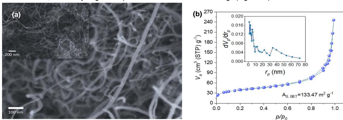
Figure 1: (a) SEM image of purified CNT from PWO and (b) N<sub>2</sub> adsorption-desorption isotherms with BJH plot
