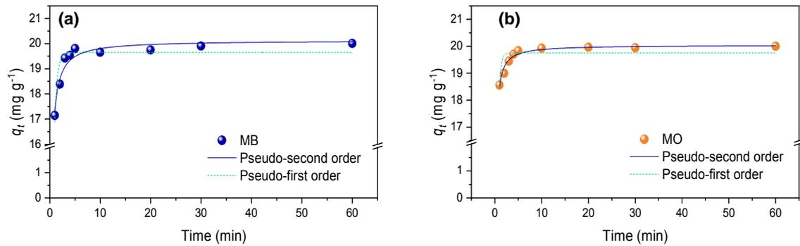
Figure 3: Time profile and kinetic model fitting of (a) MB and (b) MO adsorption in CNT at  $C_0 = 20 \text{ mgL}^{-1}$ ,  $\text{pH} = 7$ ,  $\text{S/L ratio} = 0.1 \text{ gL}^{-1}$ ,  $V = 25 \text{ mL}$ , and  $T = 25 \text{ }^\circ\text{C}$ .
